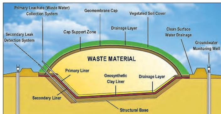
A typical cross-section of a Class 1 residual waste landfill
